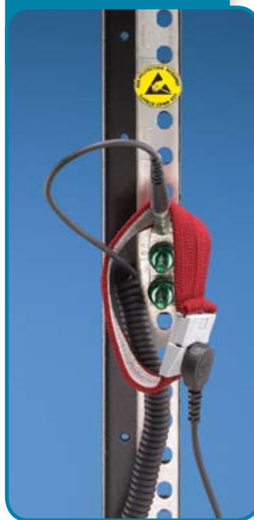
Figure 4. Electrostatic discharge wrist strap and wrist strap port.
